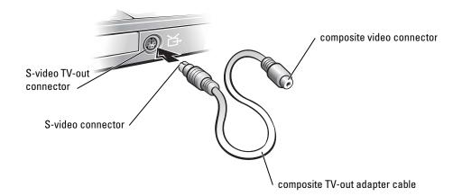
**3** Plug one end of the composite video cable in to the composite video connector on the composite TV-out adapter cable.
